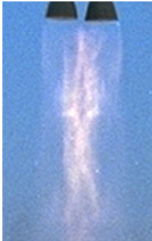
Figure 5 Visible light from the twin engines of a Titan IIB close to the Earth's surface
